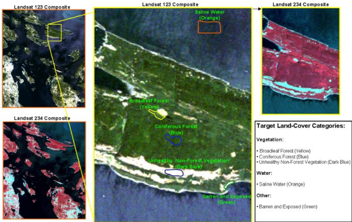
Location of basic land-cover classes focusing on Landsat TM true color (123) composite. Five classes (including Water) are presented.
